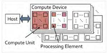
Figure 28. OpenCL architecture.
